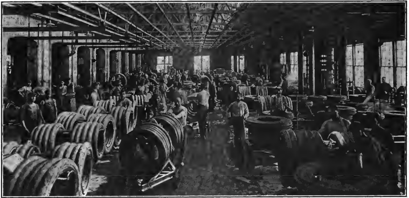
Scene in the curing room where pneumatic tires are given their first vulcanization
